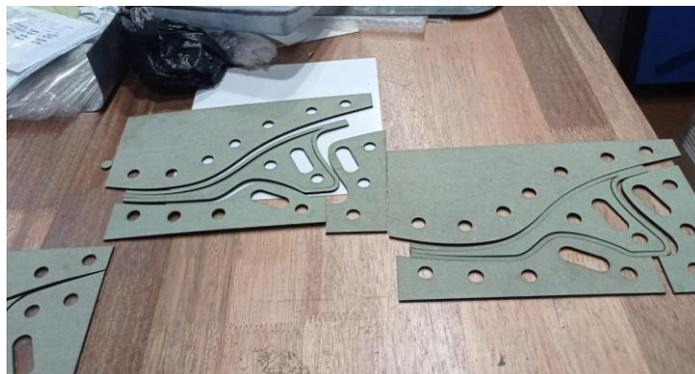
**Gambar 11.** Hasil proses *laser cutting*
